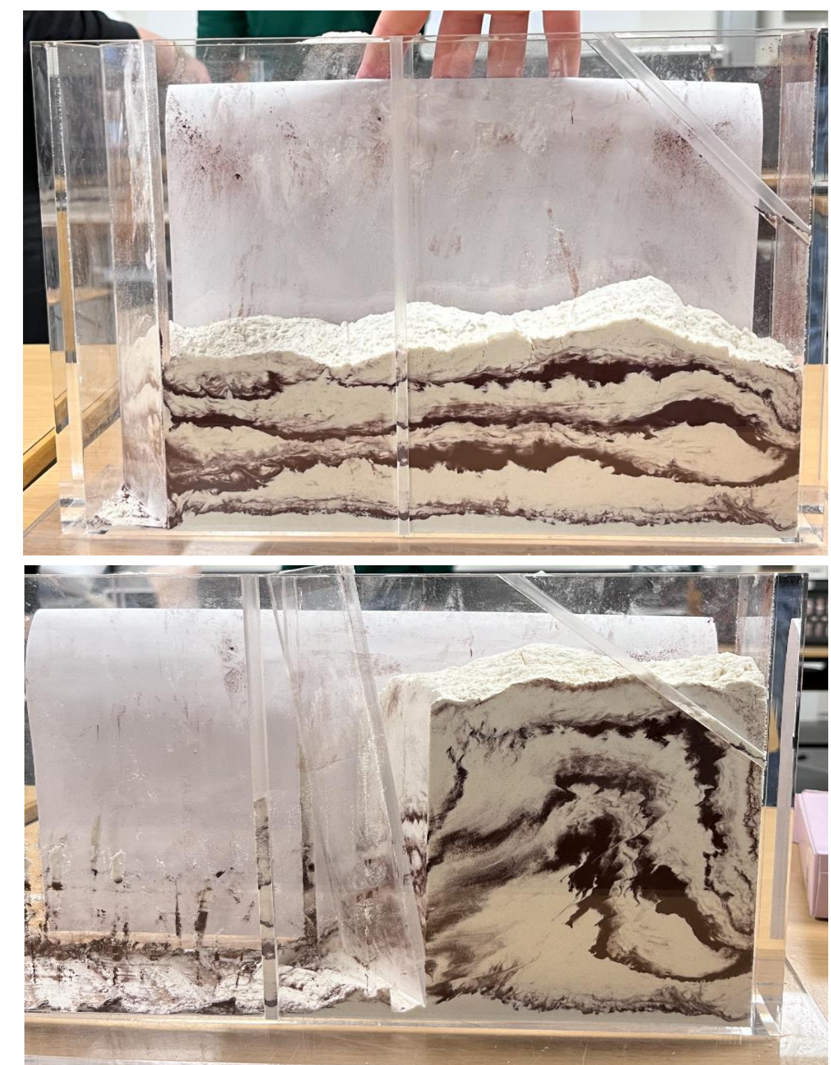
Fig. 2: A model for the formation of faults to trap the oil
