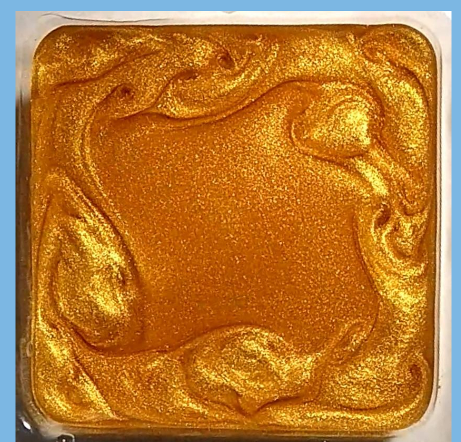
Fig. 4. A mixture of powdered mica and water rotating in a square vessel.
