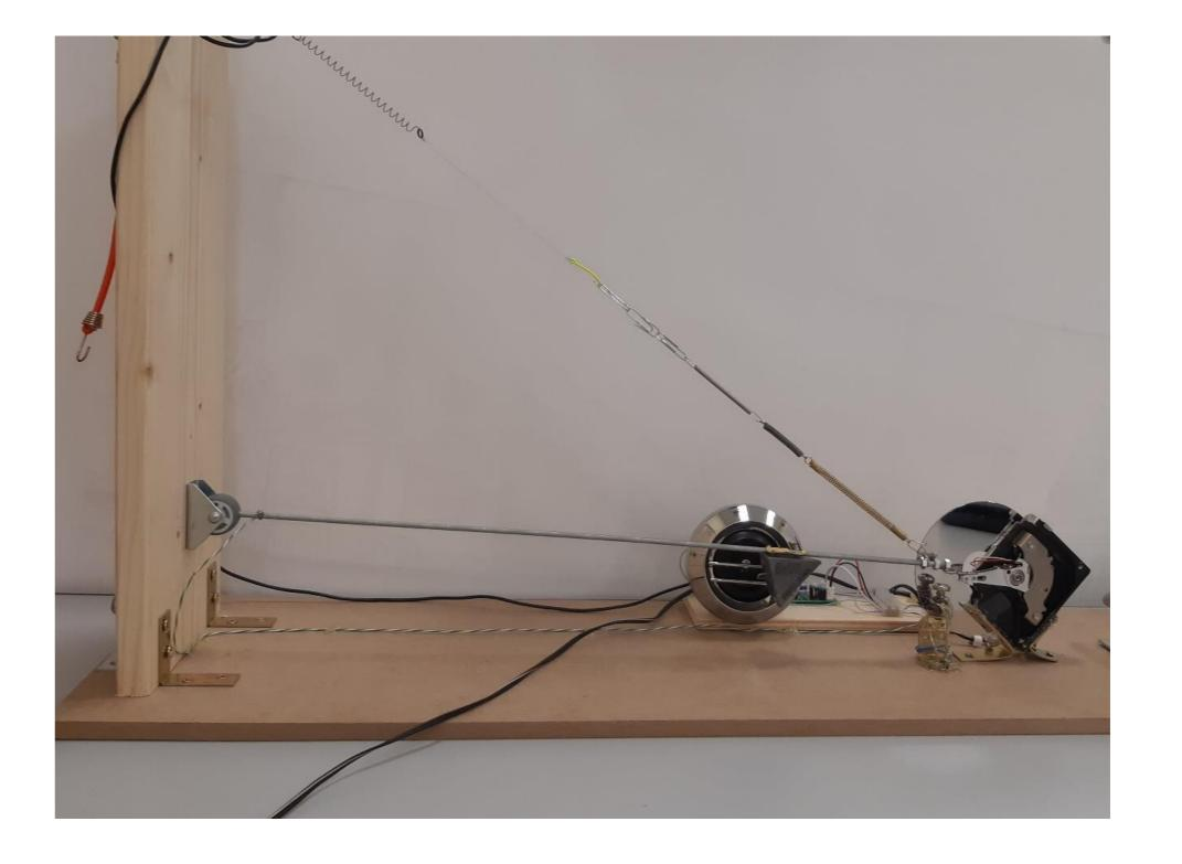
**spring system** that oscillates vertically due to vibrations.
