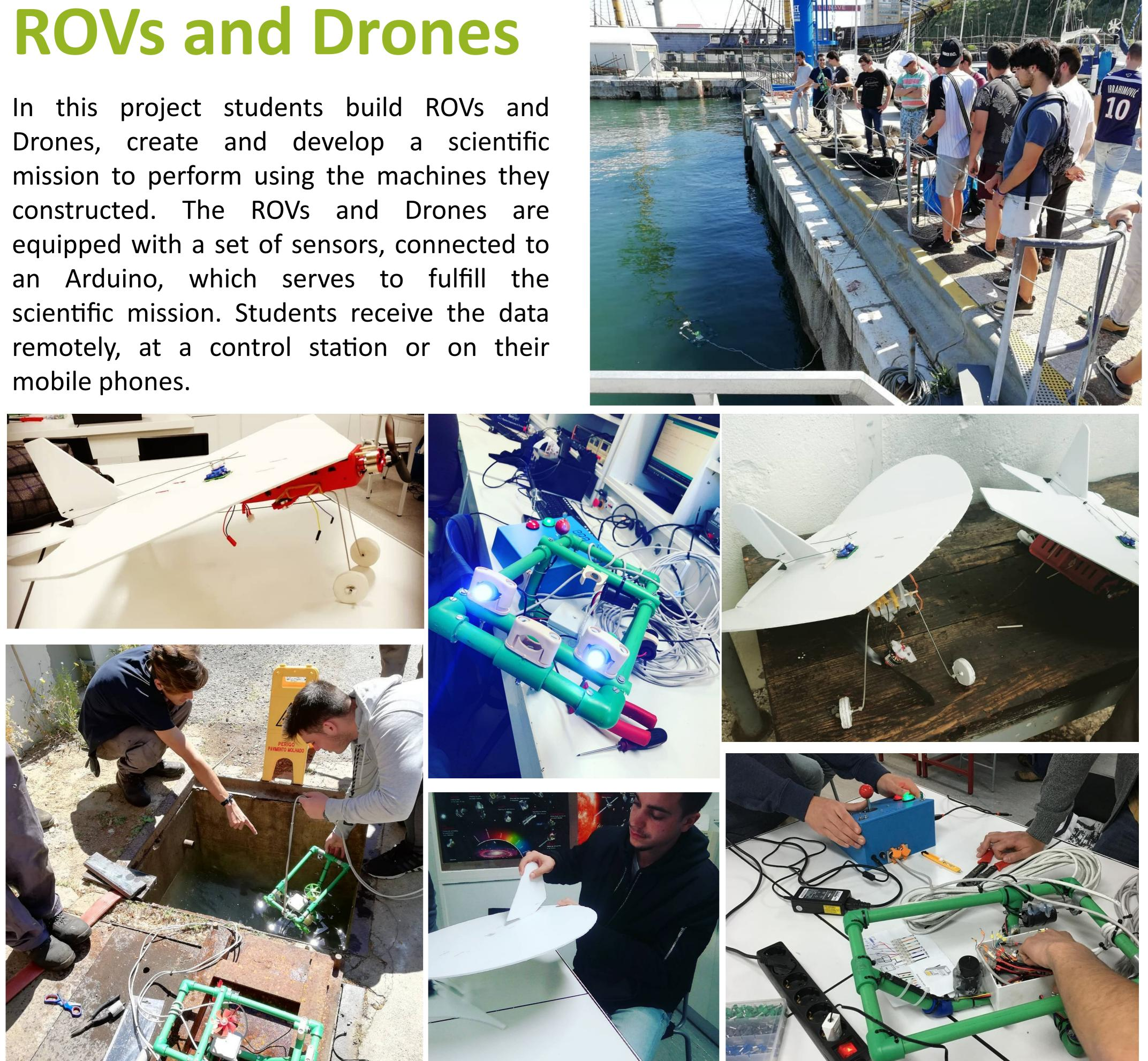
Starting from ROVs and Drones (RC Airplanes) plans that are available on the internet, students build these ROVs and Drones and add sensors, connected to an Arduino, to fulfill a scientific mission to be accomplished in water or air.
