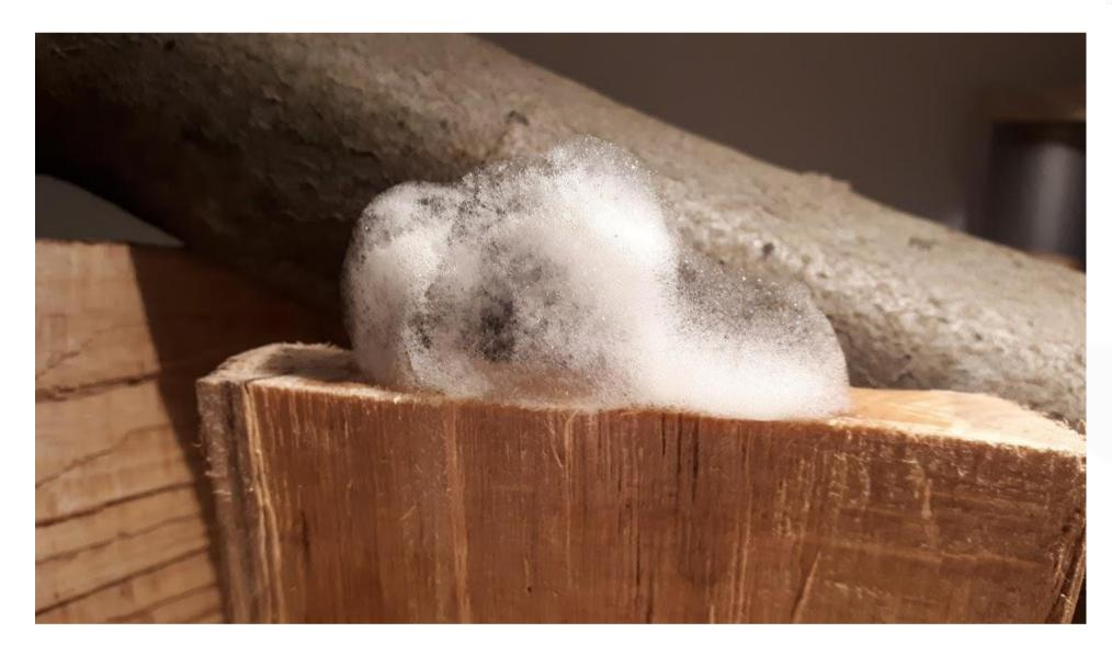
How do we know that the wood is dry? The most reliable method is using moisture measuring device or measuring density – dry wood is lighter than the wet one. Our experiment is applicable to beech firewood. water and dissolved minerals
