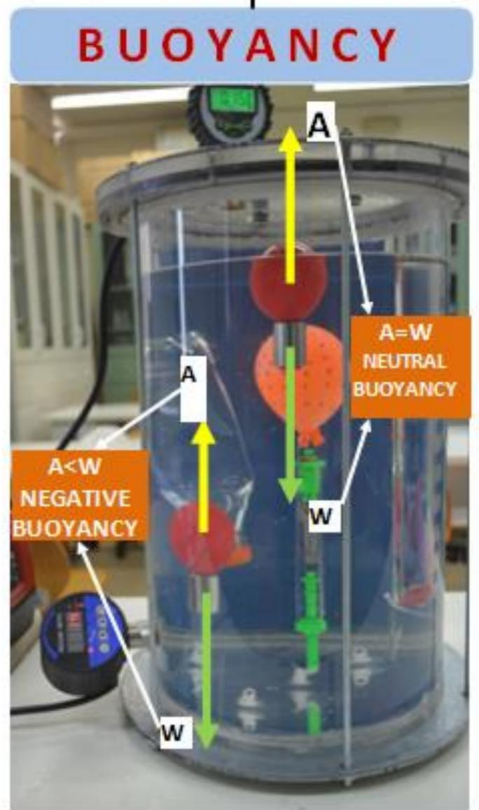
This prototype **Hyperbaric Chamber** is transparent, making it possible to present a number of principles of physics in a high pressure environment, while at the same time allow high precision measurements without a precedent.
