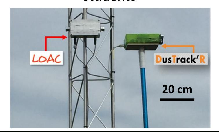
**DusTrack'R** is a versatile platform for measuring precisely air pollution in real-time based on open hardware solutions (Arduino + commercially available sensors).
