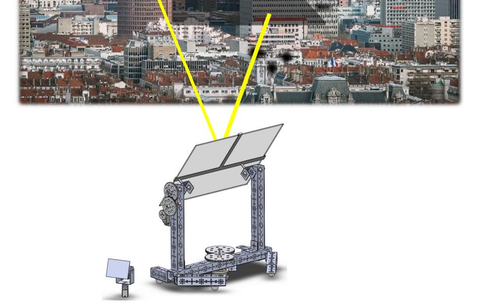
The reflected area is fixe (the room to be illuminated) but the position of the sun varies. The automatic inclination of the mirror will have to take into account these 2 parameters.
