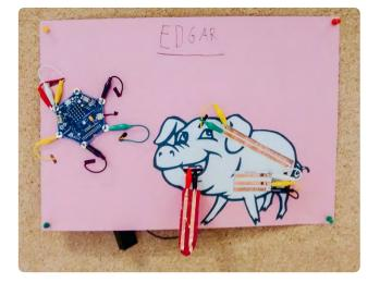
When the simulated pet feeds, taste sensors obviously cannot be used. Instead, the appropriate sensor 'reads' the offered food and the algorithm is controlled by a suitable conditional branch so that the output corresponds to the expected behaviour of the pet. Therefore, the display of the cat simulator shows a smiley (face) when it is fed a mouse and a sad face when it receives a bone. These branches are the same for both versions of the workshop.
