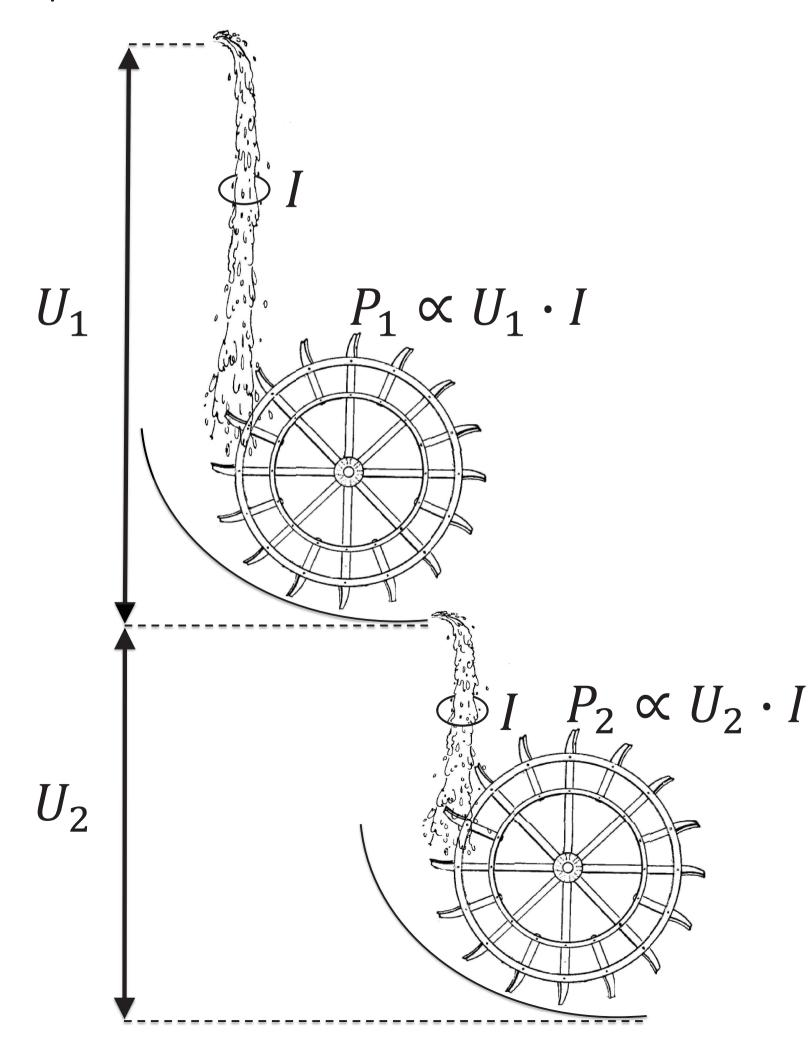
Water flowing in tubes can demonstrate all aspects of the resistance of electric wires.  $R = \rho \frac{L}{A}$
