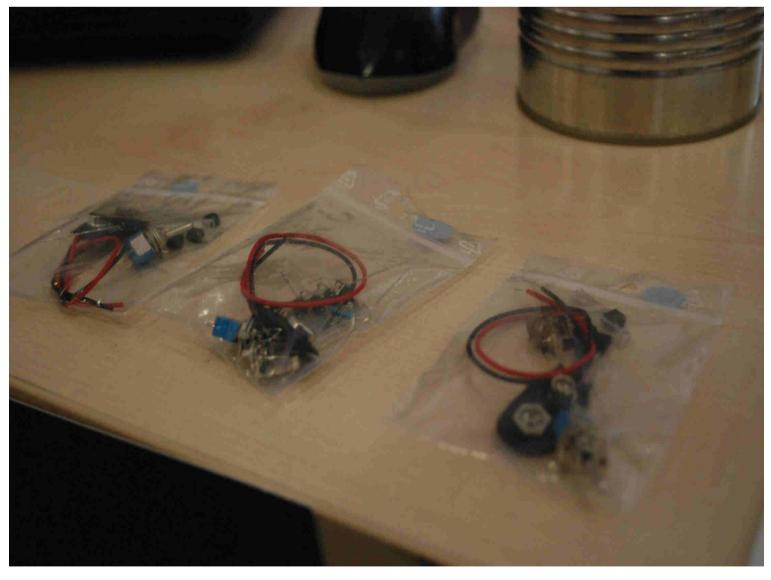
To help the DIY process, we made some kits, pre assembled amplifiers with the resistors. This action provides an easier approach if you want to build the detector. Also these kit elements are cheap and easy to get, even from scrap parts.(e.g.: old transistor radio) If you choose these kits, all you need to have, is two different sized tin cans, some aluminum foil, a multimeter, and a 9V battery. Everything else will be in the kit.
