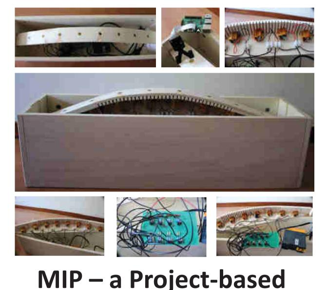
dot in our hand. The camera detects the small dot and transmits information to the board. The board, then, processes the coordinates at which the dot is in and emits a musical note through the speakers.
