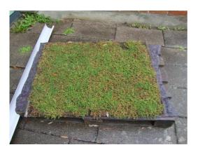
Suggestions for constructing a roof model, type "roof 1" for flow measuring unit A: Using a wooden pallet; felt with nutrients for establishing plant growth; a mat of Sedum plants; a gauge to collect rain water.
