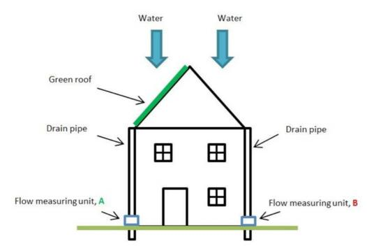
Monster rain sketch for constructing a prototype roof with two sides, one side with green plants that detain the runoff, the other side a control with no plants to absorb and delay the runoff.
