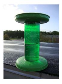
You can collect precipitation in a rain gauge – and make a rain calendar for the period of your monitoring. Note down the amount of rain every time you empty it.
