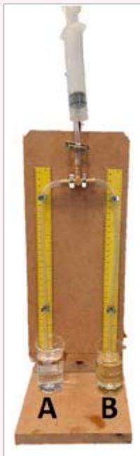
Allow several minutes for the capillary action in each tube to settle.
