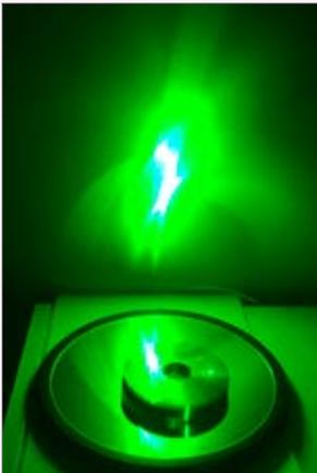
the velocity of the precession increases continually. This can be observed by the increasing frequency heard and the decreasing radius of the circular laser projection.
