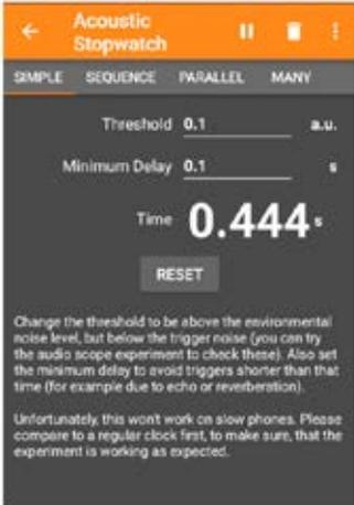
Change the threshold to be above the environmental noise level, but below the trigger noise (you can try the audio scope experiment to check these). Also set the minimum delay to avoid triggers shorter than that time (for example due to echo or reverberation).
