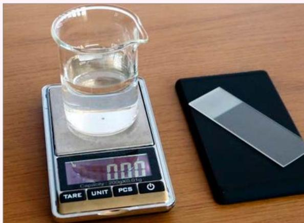
4. Convert the reading on the scales from grams weight to newtons. (Multiply by 9.8 / 1000)
