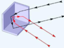
2. If the light is reflected from all three surfaces then it is inverted and rotated. Your own reflection in the three mirrors of a corner reflector will appear upside down and reversed left-to-right. (This is quite different from the reflection in just two mirrors.)
