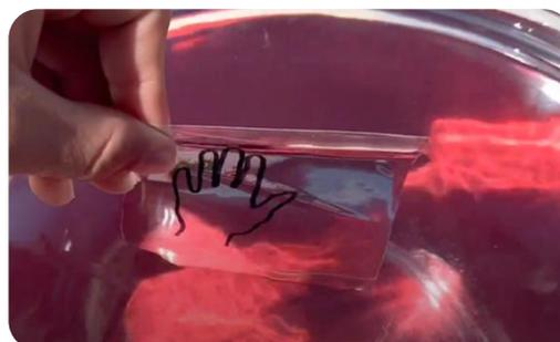
Figure 40.2: When placing the bag in water and viewing from the right angle, the drawing inside the bag becomes invisible.
