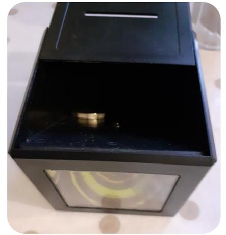
Figure 36.3: Mirror box - Note the line of the mirror at 45 degrees across the left-hand face.
