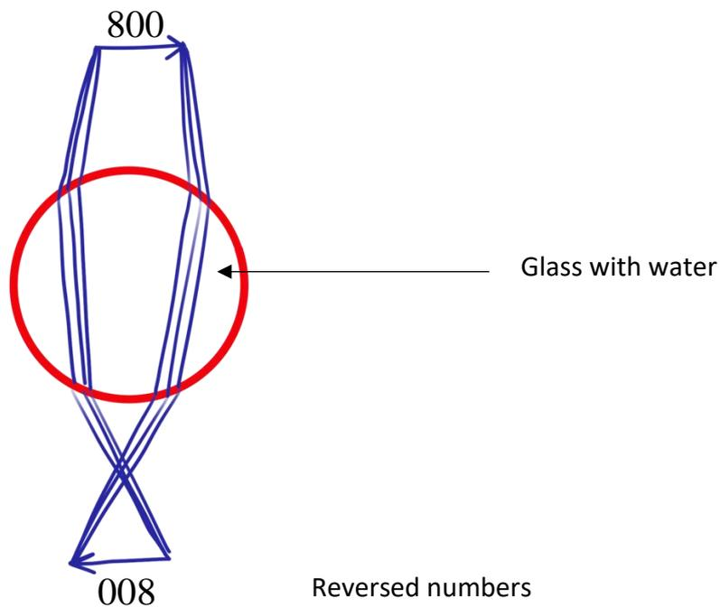
Figure 48.3 Diagram showing light refraction in a glass of water.
