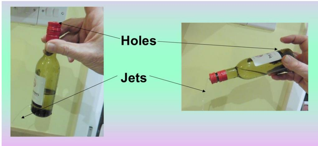
Figure 32.3: The bottle can be similarly used , with two holes. The second hole must be uncovered to release the contents of the bottle.
