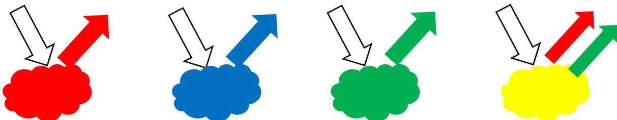
Filters absorb some light and transmit other light. So using filters to observe objects causes them to be observed in different colours.
