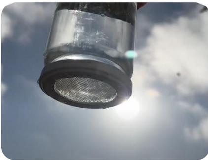
Figure 5.3: Lid with a insect mesh cut to size.
