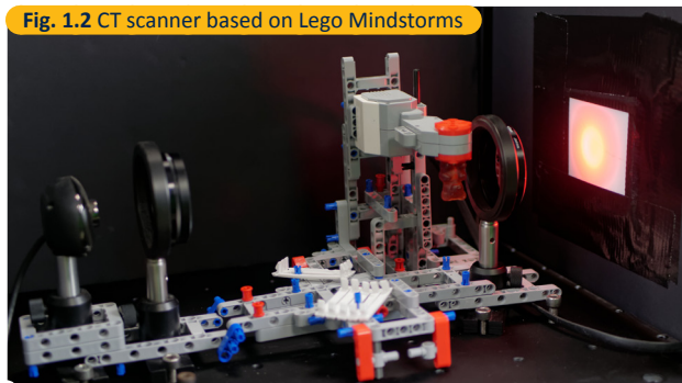
Fig. 1.2 CT scanner based on Lego Mindstorms
