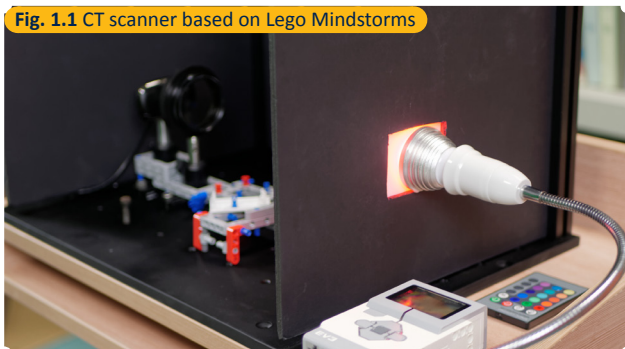
Fig. 1.1 CT scanner based on Lego Mindstorms
