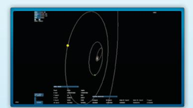
The elliptical Hohmann trajectory (dotted) follows a rotational movement following the start planet of the spaceship. The students click the HOHMANN button and wait until the ellipse stops. At that moment the spacecraft begins its journey because the planets' configuration is favourable.
