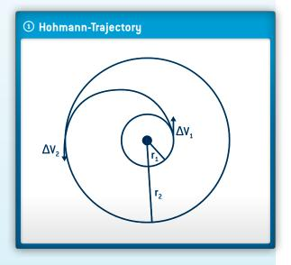
The spaceship has to change its velocity twice, once at the beginning of the elliptical trajectory, and once at the end. This is done using the so-called velocity impulse delta-v ( $\Delta$ v). This change in velocity is a measure of the "effort" that is needed to change the trajectory when performing an orbital manoeuvre.
