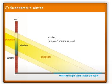
In these two pictures (0, 0), in which the wall faces toward south, we drew the inclination angles of the sunbeams at noontime. At this time, the sun reaches the maximum latitude on the horizon of a solstice day (December 21st, the winter solstice and June 21st, the summer solstice in the Northern hemisphere).
