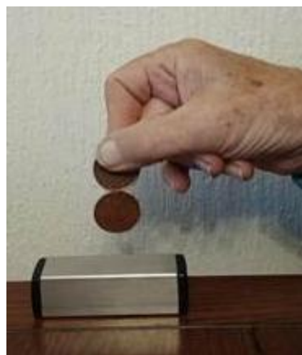
Photo 2: Induced Magnetic field holds coins together
