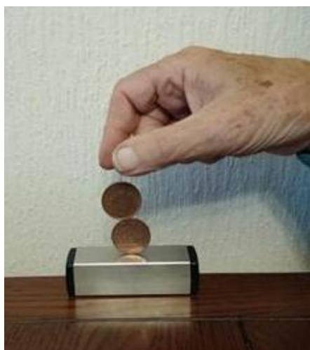
Photo 1: Induced magnetic field holds coins in position
