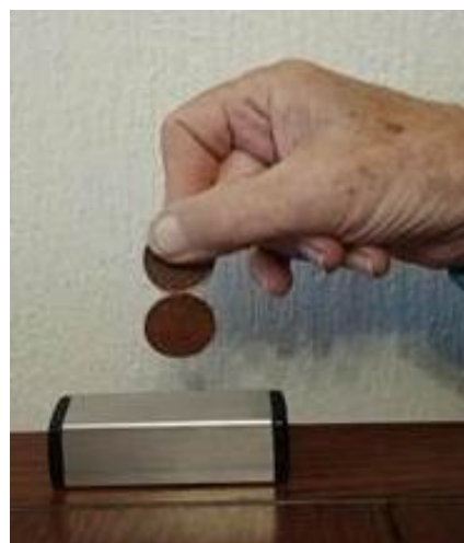
Photo 2: Induced Magnetic field holds coins together
