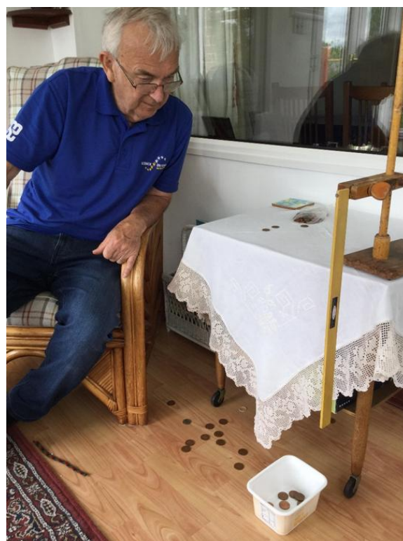
Photo 3: Note that only half of the coins reached the container, those on the floor are roughly below their starting points.
