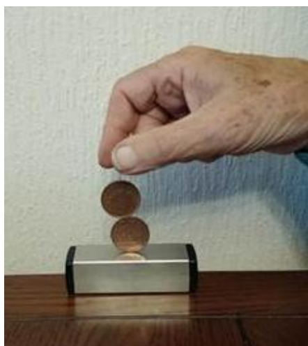
Photo 1: Induced magnetic field holds coins in position
